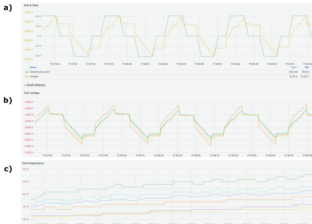
Figure 2 Sensing validation at 25 °C and 40 A where a) shows current and voltage at module level, b) shows voltage at cell level and c) shows temperatures at cell level
