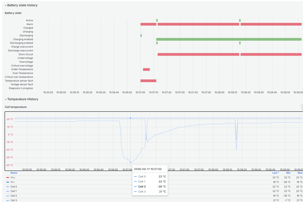
Figure 17 Under temperature alarm activation
